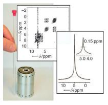
Analysis on the go: Portable high-resolution NMR spectroscopy is of great interest for many applications. Recent advances in magnet design, spectrometer stability, and acquisition schemes have placed the realization of low-field spectrometers based on room-temperature permanent magnets and that can deliver chemical shift resolution within reach.
